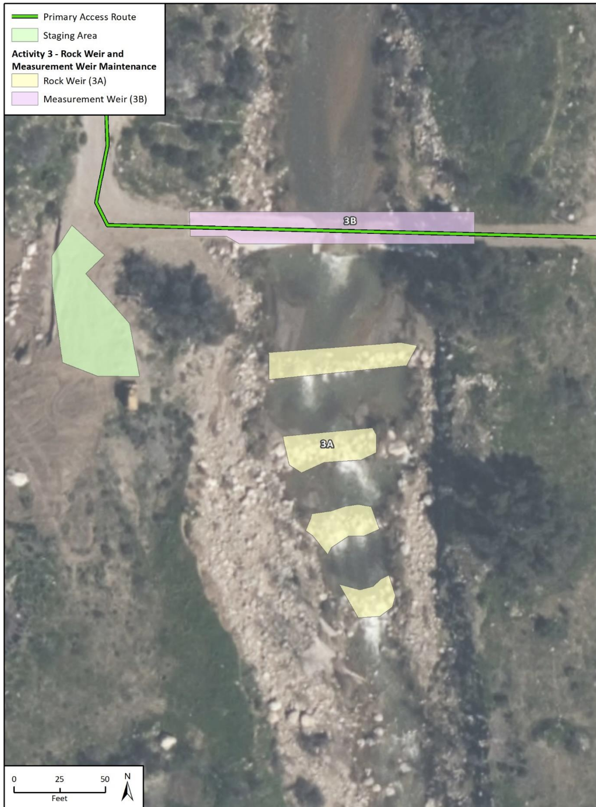
Figure 4 Activity 3 Rock Weir and Measurement Weir
