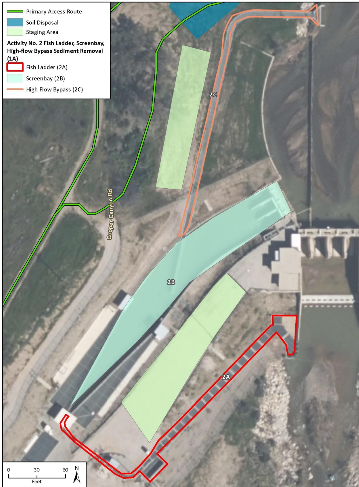
Figure 3 Activity 2 Fish Ladder, Screenbay, High-flow Bypass
