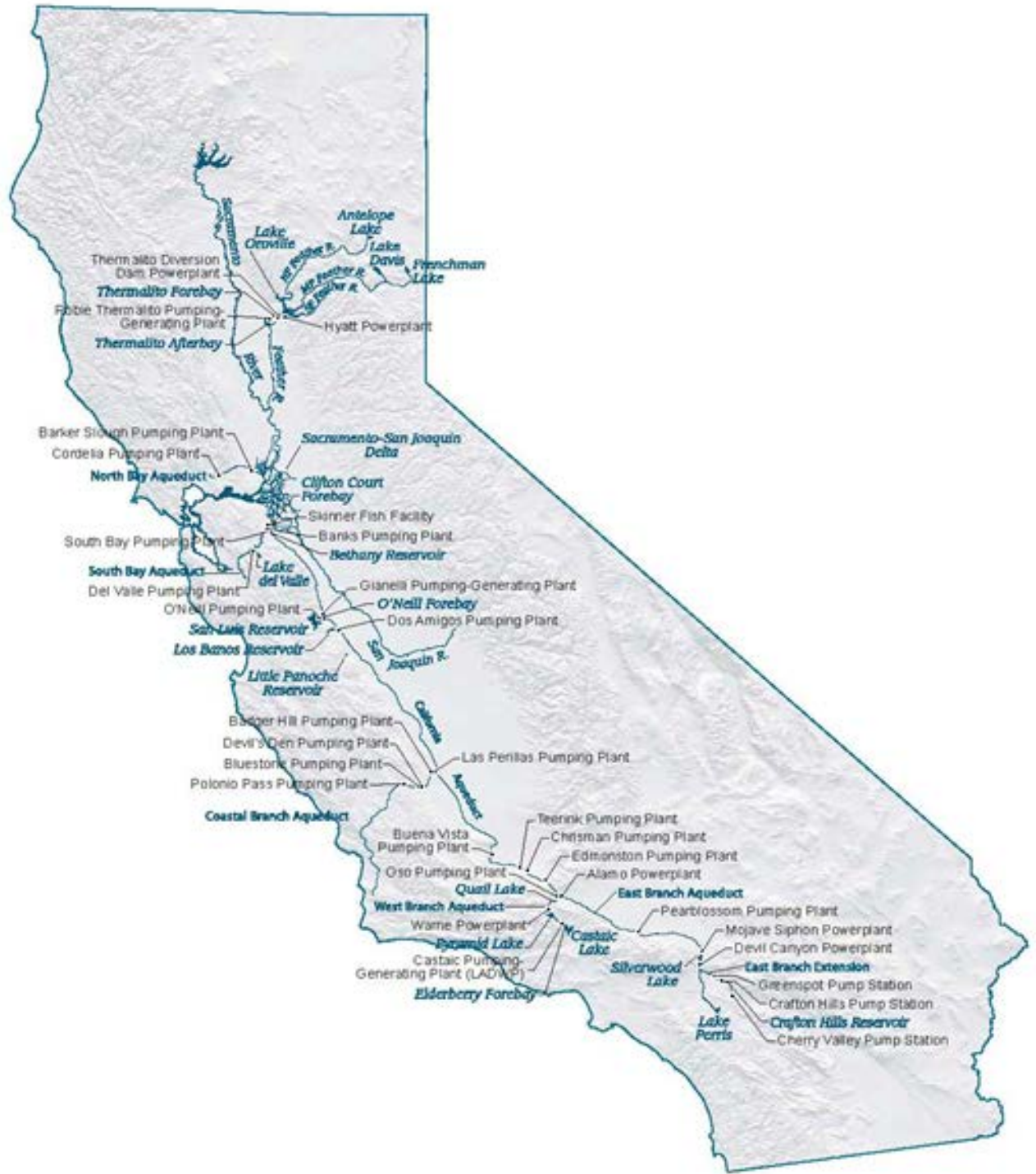
Figure 6-2 SWP Delivery Facilities
