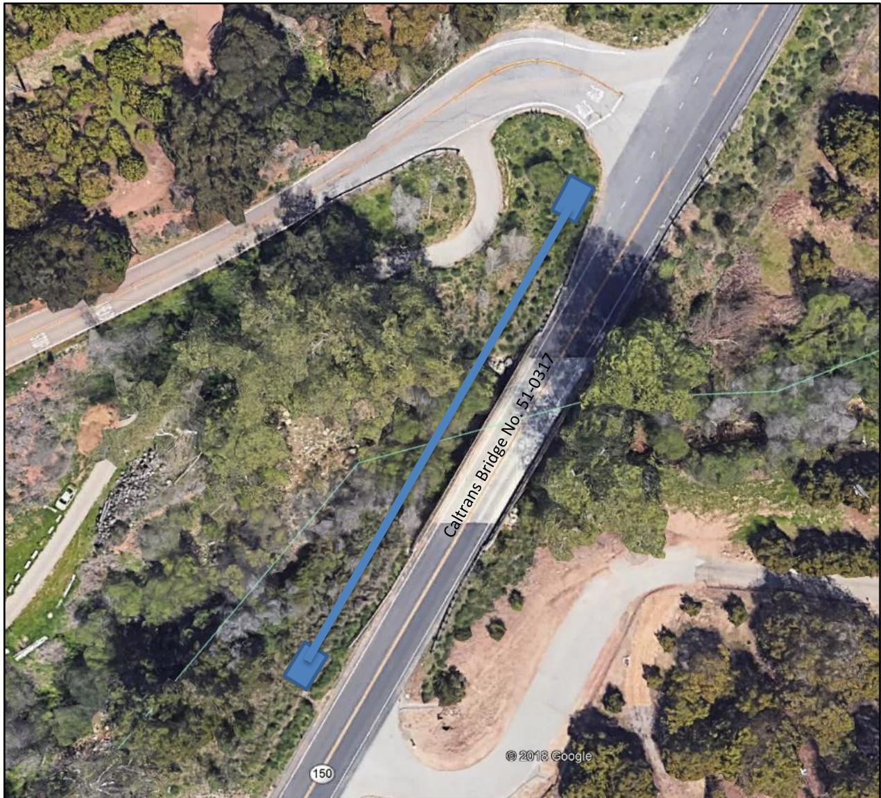
**Figure 3** – Trenchless Undercrossing Option 2C. Length approx. 300 feet. Requires deep shafts (approx. 30 to 40 ft. deep) to get below Younger Alluvium cobbles and boulders in the middle of the creek channel and safely into the underlying Casitas Formation.
