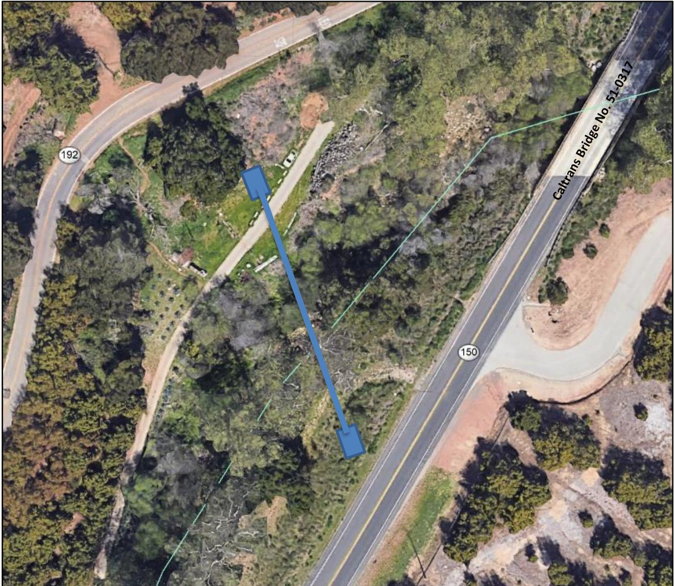
**Figure 1** – Trenchless Undercrossing Option 2A. Length approx. 240 feet. Requires deep shafts (approx. 30 to 40 ft. deep) to get below Younger Alluvium cobbles and boulders in the middle of the creek channel and safely into the underlying Casitas Formation.
