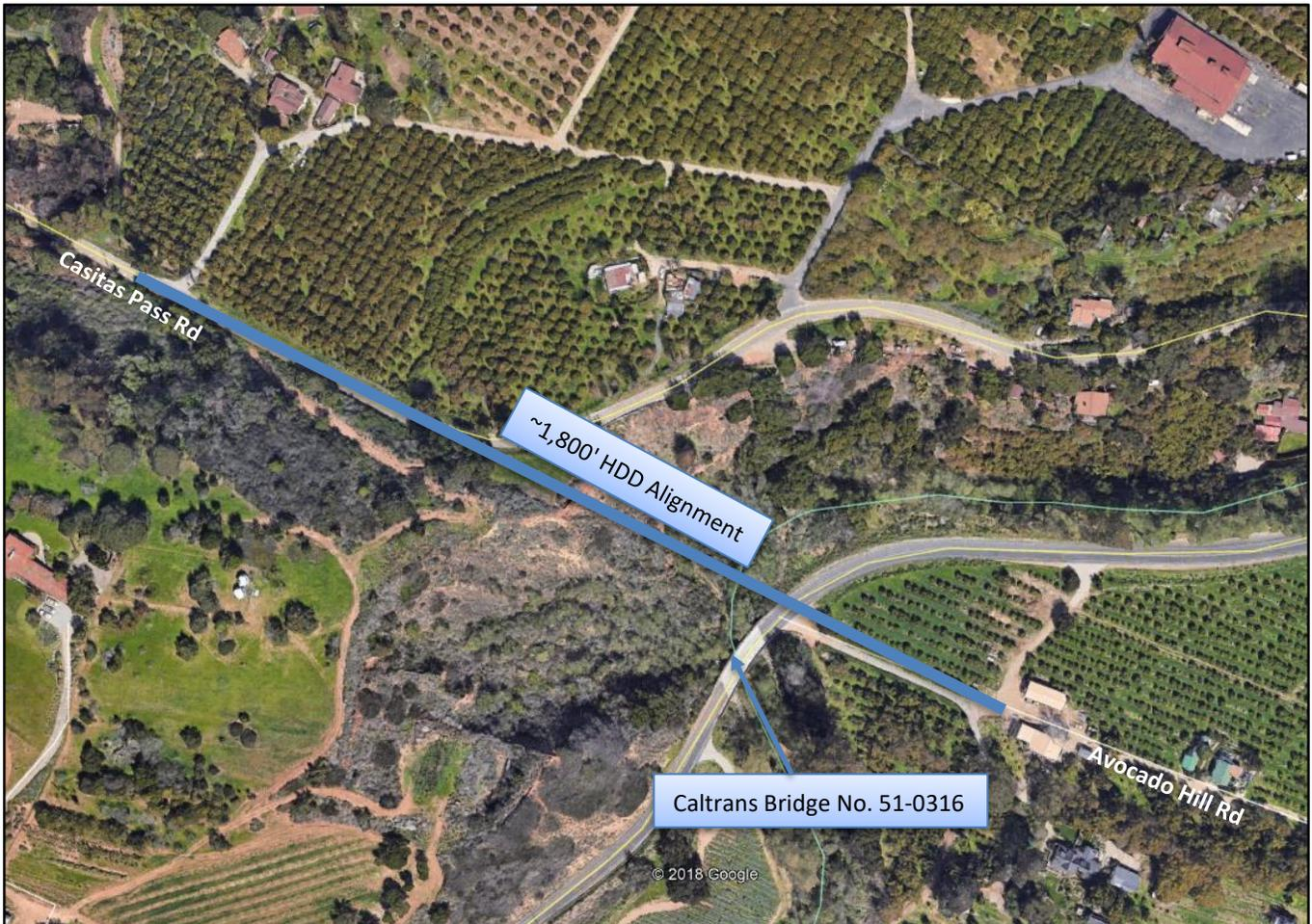
**Figure 2** – Trenchless Undercrossing Option 2B. Length approx. 1,800 feet. Requires specialized conductor casing (gate valve and rubber entry seal) on downhill (HDD entry) side to safely contain HDD drilling fluids. HDD bore path to be well within Older Alluvial Deposits and Casitas Formation.
