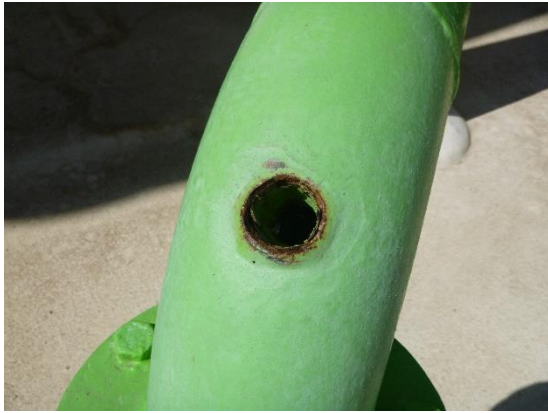
Fig. 1.7. Water feature corrosion
