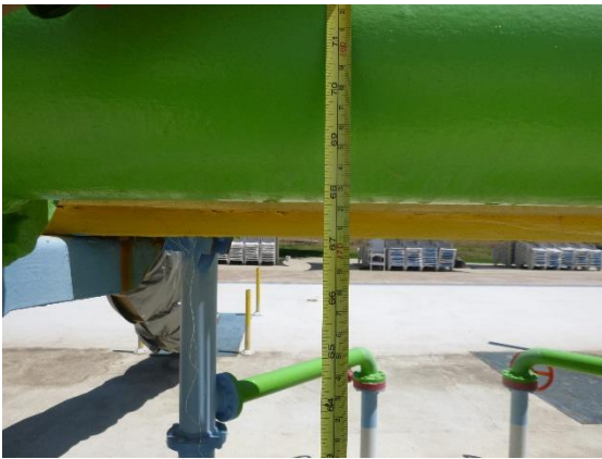
Fig. 1.19. Uneven platform connection
