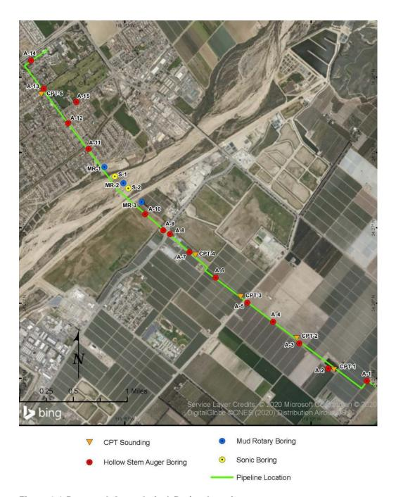
Figure 2-1 Proposed Geotechnical Boring Locations
