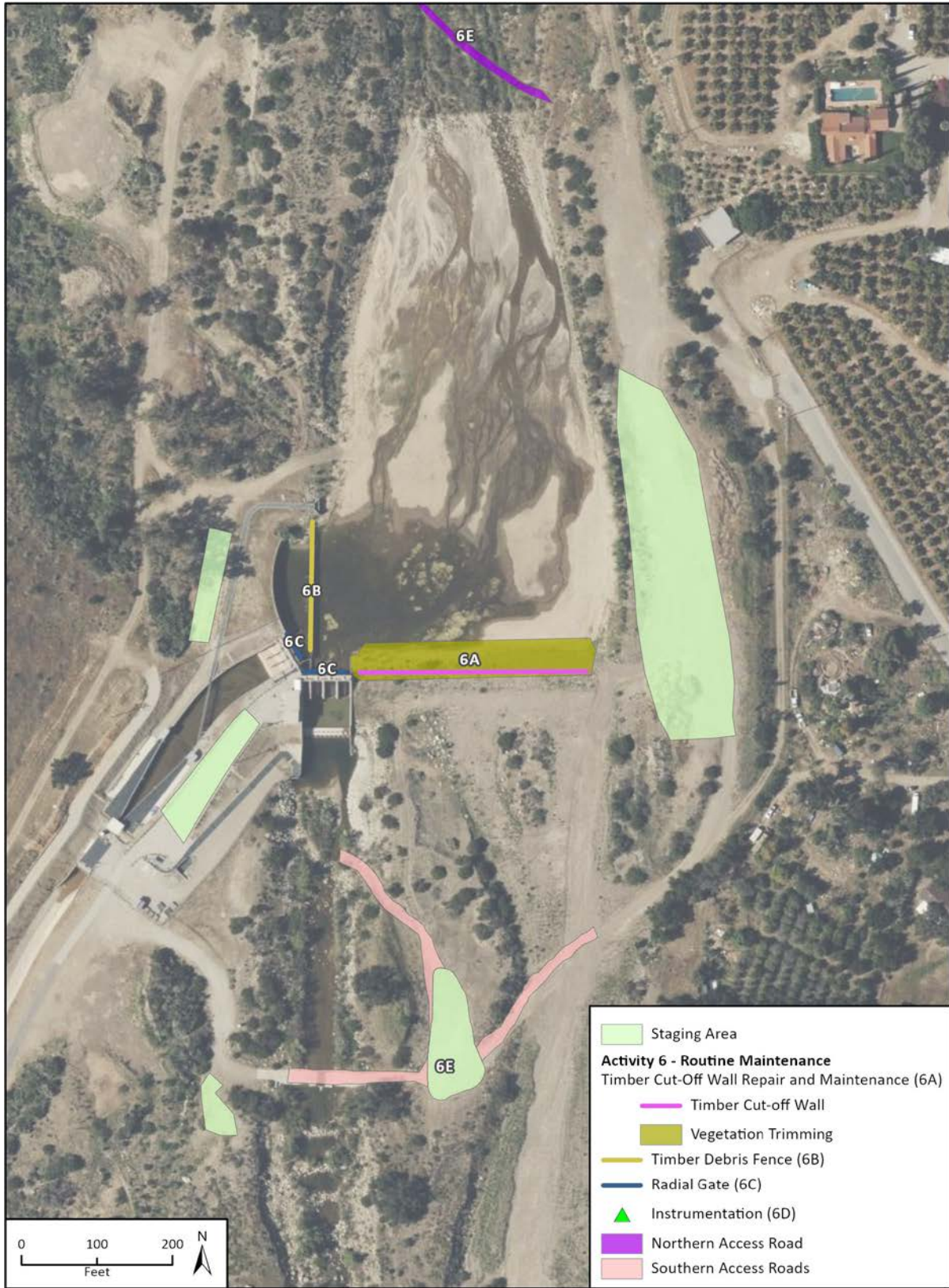
Figure 8 Activity 6 Routine Maintenance
