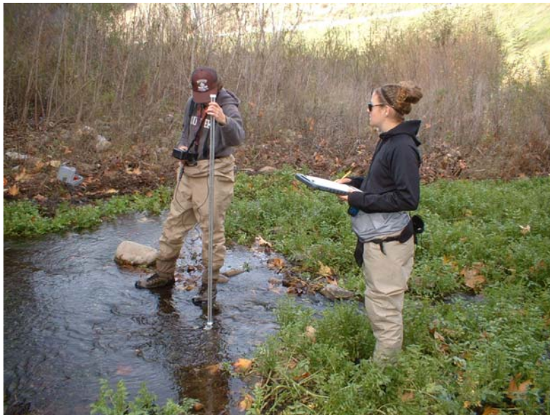
Figure 2. Photo taken during the data collection process after a redd was identified. This particular activity is demonstrating water velocity measurement.
